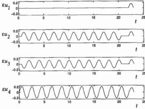
Fig. 1. Control input signals for AUV example with four controls.
