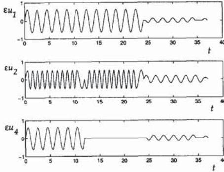
Fig. 3. Control input signals for AUV example with three controls.
